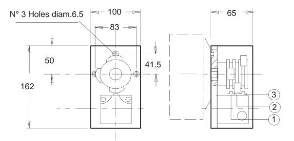
Fig. 12 - Overall dimensions of complete FC3 assembly Model and manufacturer of the multiple precision limit switch Balluff. BNS 543-B 03 R 12-61-12, or, EUCHNER SN 3-R 12-502
