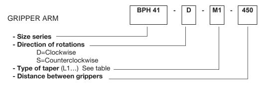
EXAMPLE: Gripper arm for BT 40 taper with gripper distance 450 [mm]
