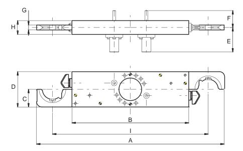
Fig. 13- Arm Gripper
