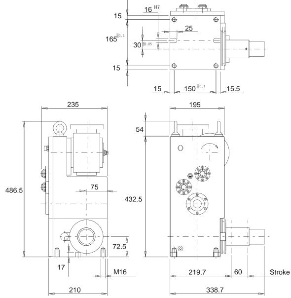
• Linear tool extraction and insertion stroke of tools is 60 (mm) is the longest achievable; upon request, tool changers with shorter stroke can be supplied.
