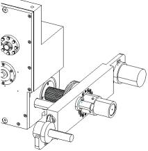
3. Extraction of Tools (output linear movement)
