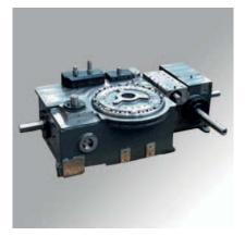
Mechanism with different cams producing seven synchronized intermittent and oscillating movements in output
