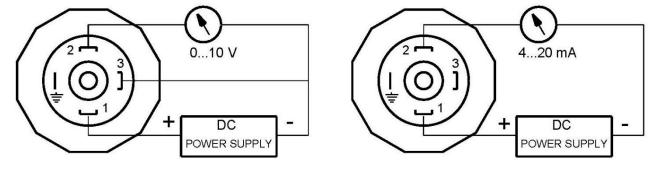
Figure 1. Transmitter connection diagram.
