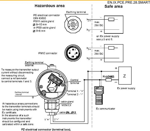
Terminals 1, 2 of the box correspond to terminals 1, 2 of the PD connector.
