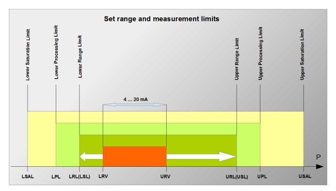
Figure 1. Set range and measurement limits.
